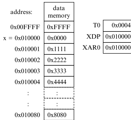
Figure 2.14 Data memory and registers
